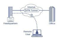
VPN Supports IPsec and SSL VPN protocols for encrypted remote access to local area network (LAN) resources over the internet.
