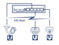
**PoE++** A 240 watt PoE power budget supplies up to four Power over Ethernet devices with PoE (15.4W), PoE+ (30W), or PoE++ (90W) power.
