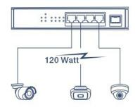
**PoE Power** A 120W PoE+ power budget supplies up to four Power over Ethernet devices with PoE+ power.
