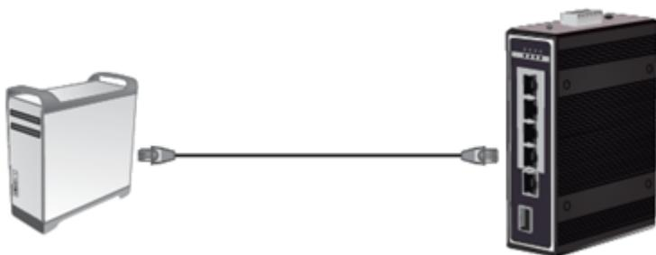
2. On your computer, run the terminal emulation program (ex. HyperTerminal, TeraTerm, Putty, etc.) and set the program to use the Telnet protocol and enter the IP address assigned to the switch. The default IP address of the switch is 192.168.10.200 / 255.255.255.0.
