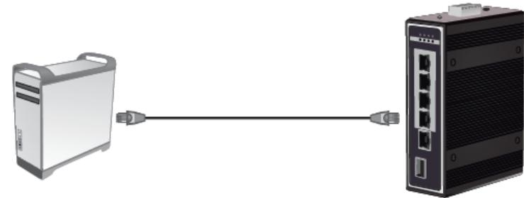
2. Assign a static IP address to your computer's network adapter in the subnet of 192.168.10.x (e.g. 192.168.10.25) and a subnet mask of 255.255.255.0.
