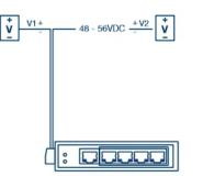
Fault Tolerance The industrial switch features redundant power inputs for backup power with overload current protection.
