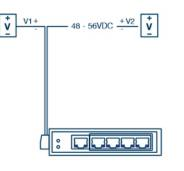
Fault Tolerance The industrial switch features redundant power inputs for backup power with overload current protection.
