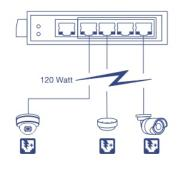
**PoE Power** A 120W PoE+ power budget for up to four Power over Ethernet devices with PoE+ power.
