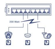
**PoE+ Power** A 200W PoE+ power budget supplies up to eight Power over Ethernet devices with PoE+ power.
