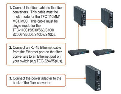
Note: The TX and RX cables must be reverse on the opposite fiber connection.
