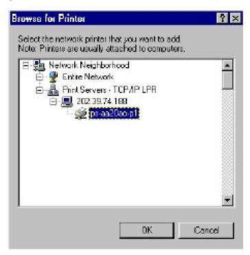
**Step 5.** Click on **Next**. If you are unable to do this you can manually enter the Print Server by using two backlashes, the IP address, one backlash and the port name of you printer.
