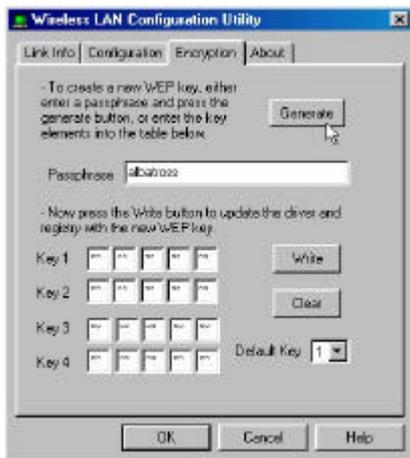
The Encryption window enables you to create an encryption scheme for Wireless LAN transmissions. Enter a "Passphrase" and press Generate to automatically generate a 64- or 128-bit key (selected from the WEP drop-down menu in the Configuration screen).
