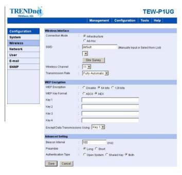
You can now input the SSID and Channel or you can click on "Site Survey". If you are using WEP Encryption, select the type of encryption and key in the value in Key 1 and click "Save".
