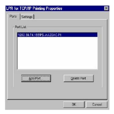
In the top field type in the IP address of your print server. In the bottom field type in the port name of your print server, the Port Name is the PS-xxxxxx-P1. X being the actual number listed in the Port Name box. Click on **OK**.
