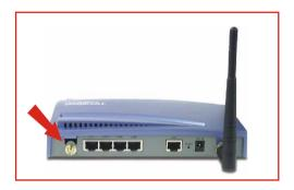
**2.** Take the TEW-IA04O connector and connect it to either your Wireless Access Point, Router, or Wireless Card.
