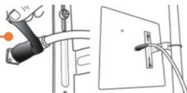
7. Connect the grounding wire to a grounding object (e.g. Earth Driven rod, Grounded Electrical System, Building Frame).
