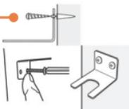
3. Loosen the nut and washer. Mount the TEW-ASAL1 on the L-bracket. Then tighten the nut and washer to secure the TEW-ASAL1 to the L-bracket.
