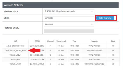
4. Click on the wireless network you would like to connect. The information will automatically fill on the previous screen. You will then need to select and enter the wireless security.
