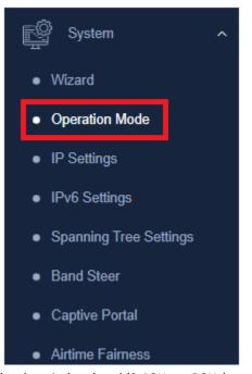
Enable Repeater, under the wireless band (2.4GHz or 5GHz) you would like to connect this access point to, then press Save. Please make sure that the selected band is available on your network.
