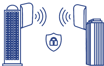
Wireless Distribution System (WDS)
