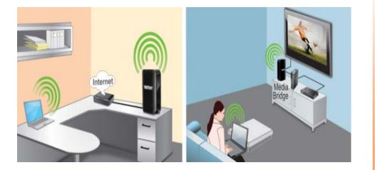
The router is installed near the modem typically supplied by your ISP "Internet Service Provider. The router's WAN port is physically connected to the modem's network port which connects to the Internet. Wireless signals from the router are broadcasted to wireless clients such as laptops (with wireless capability) thereby providing Internet access throughout your network.
