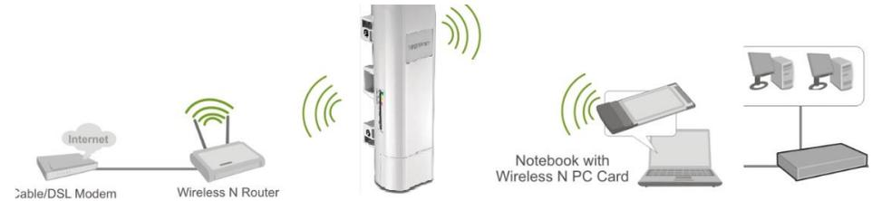
AP Repeater mode allows the access point to repeat a wireless signal of an existing wireless network. This section outlines available management options when the device System Setting is set to **Bridge** and the wireless Operation Mode is set to **AP Repeater**. Click **Apply** to save any changes.
