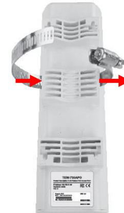
3. Align the access point to the pole and tighten up the clamp till the access point is secured on the pole.
