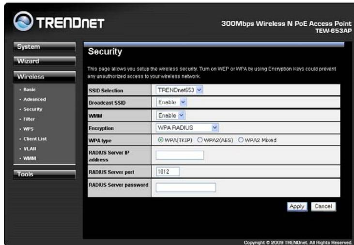
**ESSID Selection:** As this device supports multiple SSIDs, it is possible to configure a different security mode for each SSID (profile). Select an SSID from the drop-down list.
