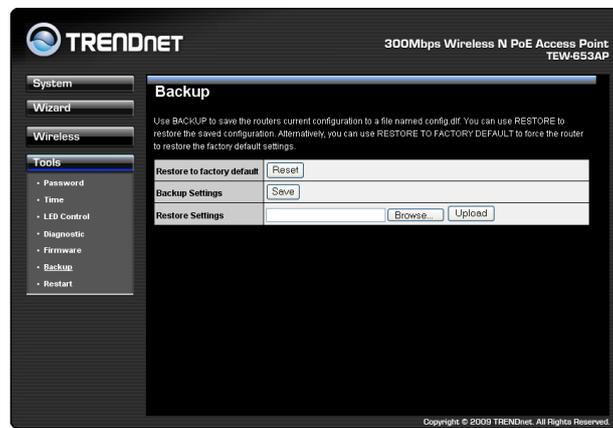
**Backup Settings:** This can save the current configuration to a file named "**config.bin**" on your PC. You can also use the **Upload** button to restore the saved configuration to the Broadband router. Alternatively, you can use the "**Restore to Factory Defaults**" tool to force the Broadband router to perform a power reset and restore the original factory settings.
