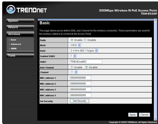
**Radio:** To enable/disable radio frequency.
