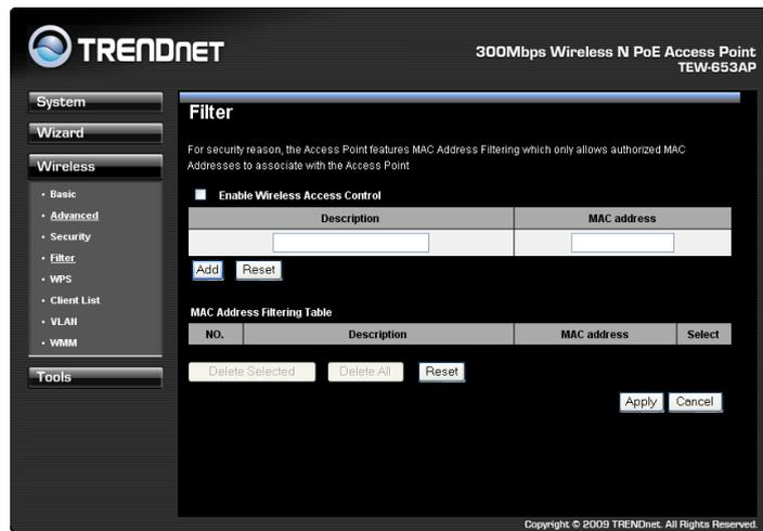
**Enable Wireless Access Control:** Check box to enable feature
