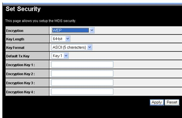
**Key Length:** Select a 64-bit or 128-bit WEP key length from the drop-down list.
