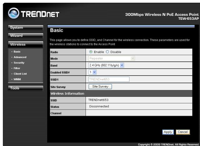
**Radio:** To enable/disable radio frequency.
