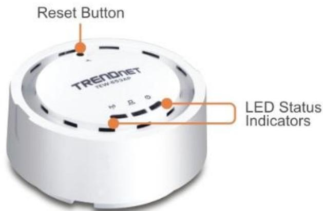
**Reset Button:** This button will reset the TEW-653AP to its factory default settings. To do this, press and hold the Reset button for 10seconds.
