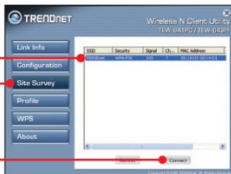
5. If encryption is enabled on your wireless network, the proper **Authentication** type and **Encryption** type will be selected automatically. Enter the encryption key and click **Apply**.
