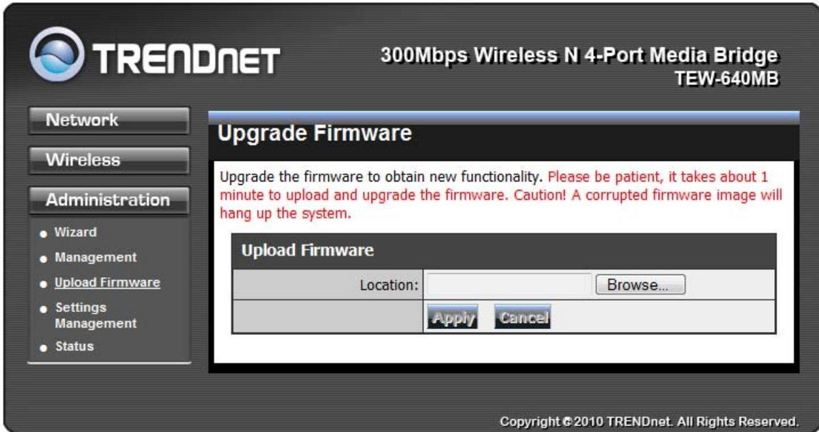
Once you have a firmware saved on your computer, use this option upload the firmware. Click on **Browse** and select the firmware file, then click **Apply** to upload the file into the adapter.
