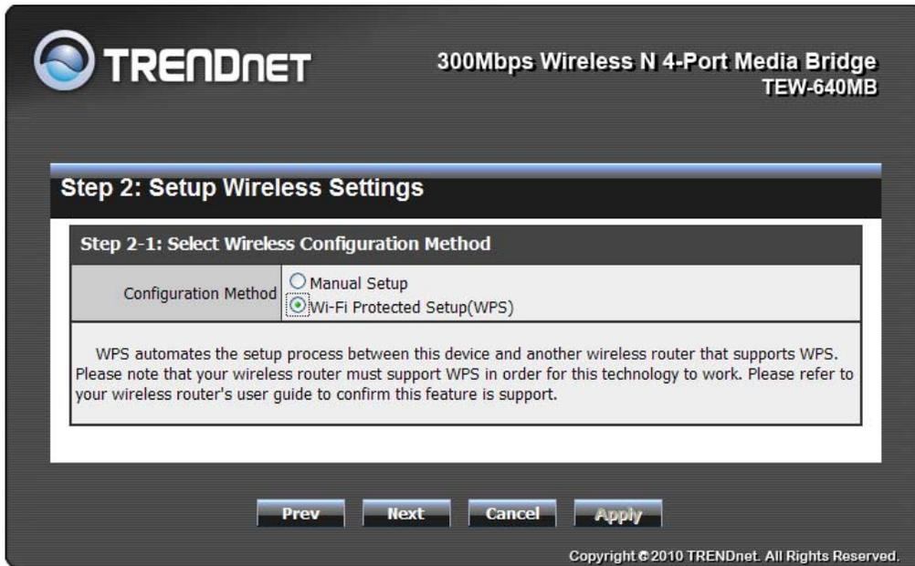
2. Select the type of WPS configuration type you would like to use. PIN configuration requires you to input the TEW-640MB PIN information into your wireless router or AP (Access Point). Click **Scan** button to select an AP SSID that you want to connect and enter Device PIN into AP.
