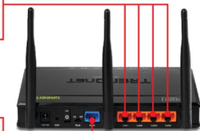
5. Connect one end of a network cable to the TEW-639GR's WAN port. Connect the other end of the cable to your modem's network port.
