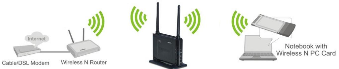
To repeat Wireless N Router’s signal, enter its wireless MAC address into “Repeater MAC Addr.” field
