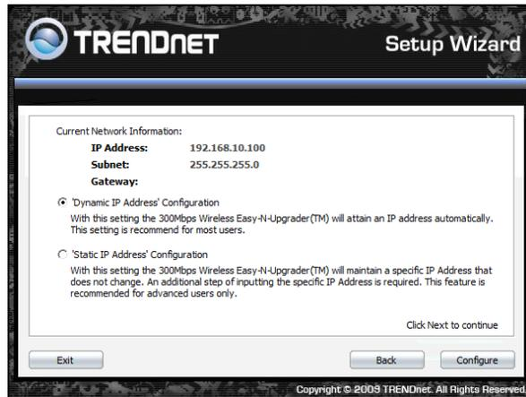
12. The default IP address is 192.168.10.100, you can choose to obtain network setting automatically, or set the IP address manually. After setting, click **Next** to continue.
