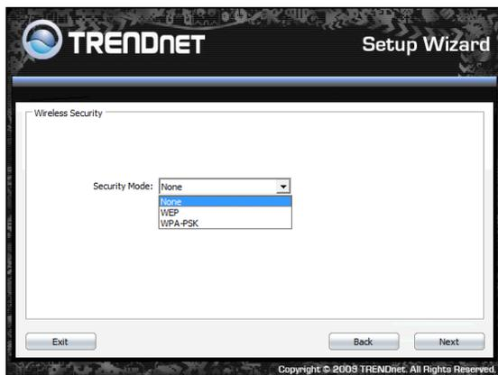
20. To use WEP security, select **WEP** and click **Next** button. Select **64-bit** or **128-bit** WEP key length, and enter your WEP key. For 64-bit encryption, enter 10 hexadecimal characters, For 128-bit encryption, enter 26 hexadecimal characters. Click **Next** to continue the setting.
