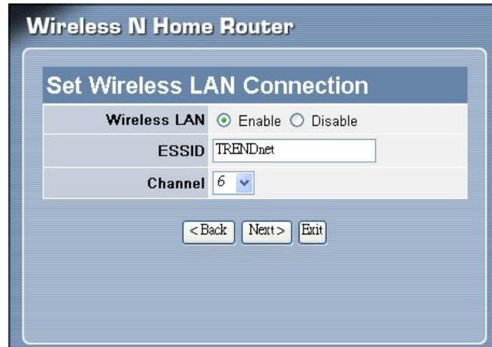
The screenshot shows the 'Wireless N Home Router' interface with the 'Set Wireless LAN Connection' page. The 'Wireless LAN' section has 'Enable' selected. The 'ESSID' field contains 'TRENDnet' and the 'Channel' dropdown is set to '6'. Navigation buttons '< Back', 'Next >', and 'Exit' are visible at the bottom.
