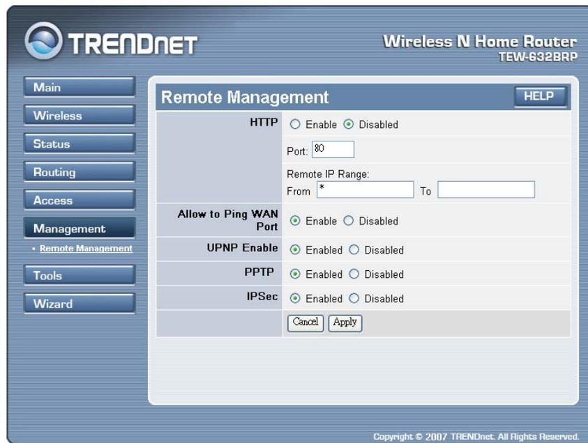
**HTTP:** Enables users to set up HTTP access for remote management.
