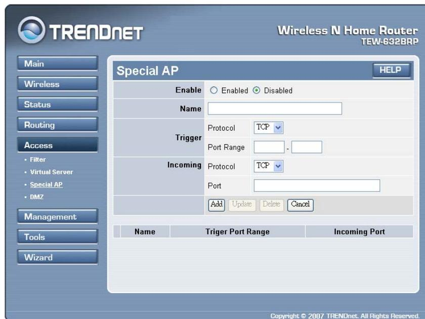
**Enable:** Click to enable or disable the application profile. When enabled, users will be able to connect to the application via the WLAN Router's WAN connection. Click "Disabled" on a profile to prevent users from accessing the application on the WAN connection.
