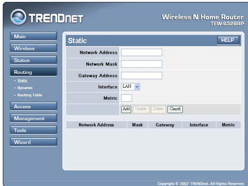
The screenshot shows the TRENDNET Wireless N Home Router (TEW-632BRP) web interface. The left sidebar contains navigation buttons: Main, Wireless, Status, Routing (selected), Access, Management, Tools, and Wizard. Under the Routing button, there are sub-options: Static (selected), Dynamic, and Routing Table. The main content area is titled 'Static' and includes a 'HELP' button. It contains the following fields and controls:
