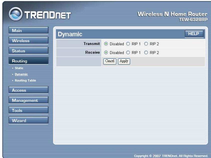
**Transmit:** Click the radio buttons to set the desired transmit parameters, Disabled, RIP 1, or RIP 2.
