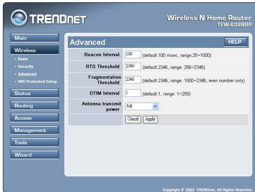
**Beacon Interval:** Type the beacon interval in the text box. User can specify a value from 25 to 1000. The default beacon interval is 100.
