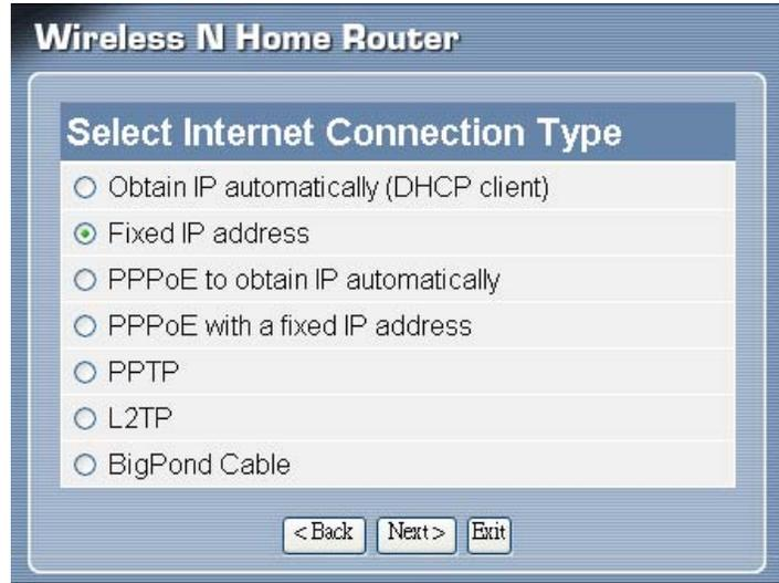
If the Internet Service Provider (ISP) assigns a fixed IP address, choose this option and enter the assigned WAN IP Address, WAN Subnet Mask, WAN Gateway Address and DNS Server Addresses for the WLAN Router.
