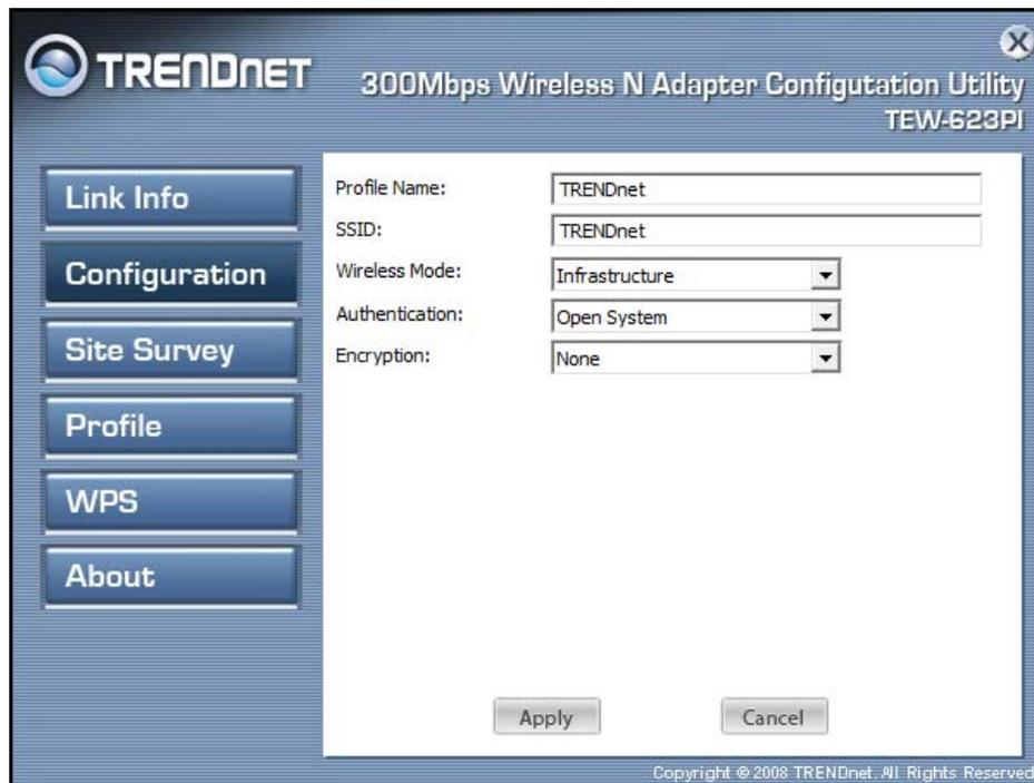
**SSID:** Service Set Identifier, which is a unique name shared among all clients in a wireless network. The SSID must be identical for each client in the wireless network.
