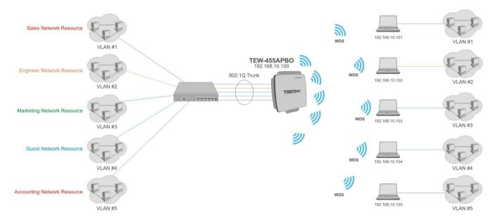
Figure 4-2 Point to Multiple Points with different VLAN Tag
