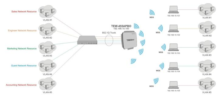
Figure 3-3 Point to Multiple Points with different VLAN Tag
