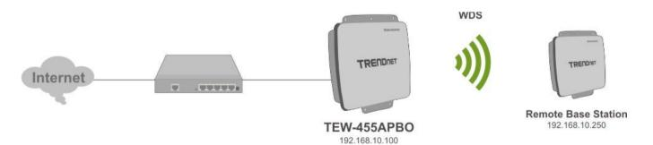
Figure 4-1 Point to Point Configuration
