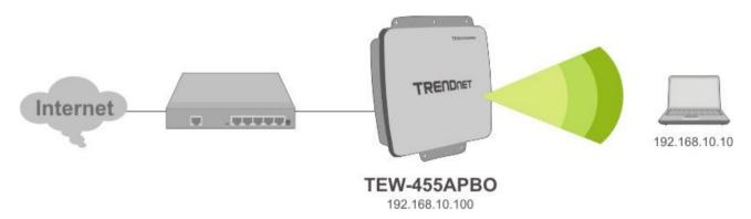
Figure 3-1 Access Point on a Wired LAN Configuration
