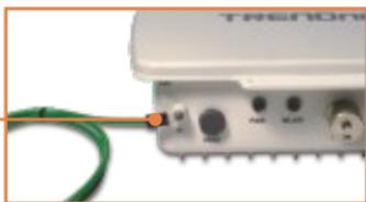
3. Connect the green grounding wire to a grounding object.
