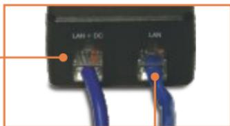
12. Connect one end of another Ethernet cable to the **LAN** port.
