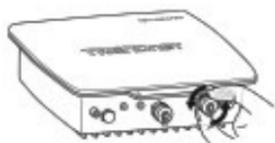
2. Screw one end of the TEW-ASAL1 to the EXT connector on the TEW-455APBO.
