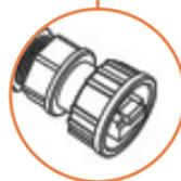
10. Connect the clamp ring and seating nut to the PoE port on the rear of the TEW-455APBO.
