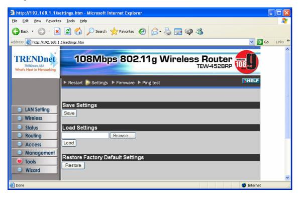
**Save Settings:** Click to save the current configuration as a profile that you can load when necessary.
