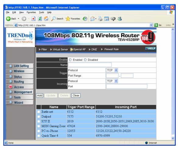
**Enable:** Click to enable or disable the application profile. When enabled, users will be able to connect to the application via the router WAN connection. Click Disabled on a profile to prevent users from accessing the application on the WAN.
