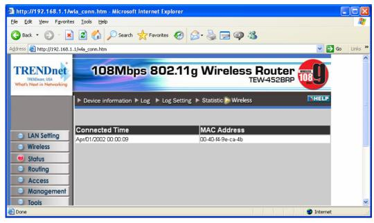
Connected Time: Displays how long the wireless device has been connected to the
