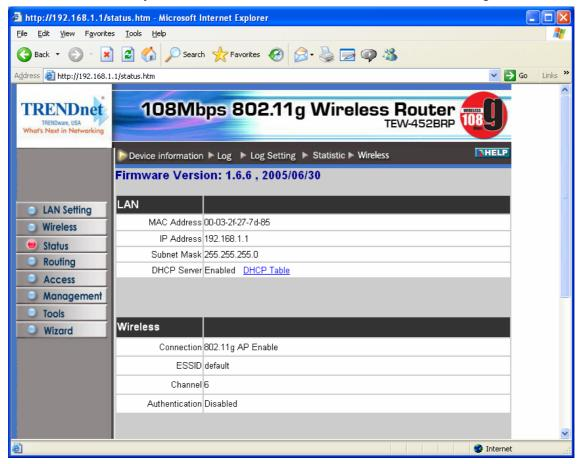
**Firmware Version:** Displays the latest build of the router firmware interface. After updating the firmware in Tools - Firmware, check this to ensure that your firmware was successfully updated.
