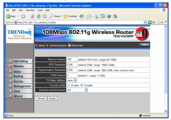
**Beacon Interval:** Type the beacon interval in the text box. You can specify a value from 1 to 1000. The default beacon interval is 100.
