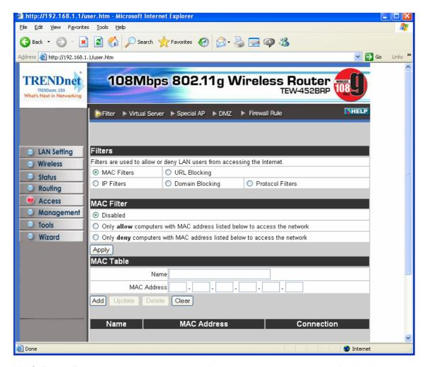
**MAC Filter:** Enables you to allow or deny Internet access to users within the LAN based upon the MAC address of their network interface. Click the radio button next to *Disabled* to disable the MAC filter.
