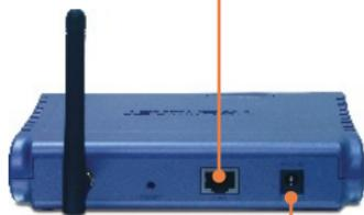
2. Connect the AC Power Adapter to the Access Point and then to a power outlet.
