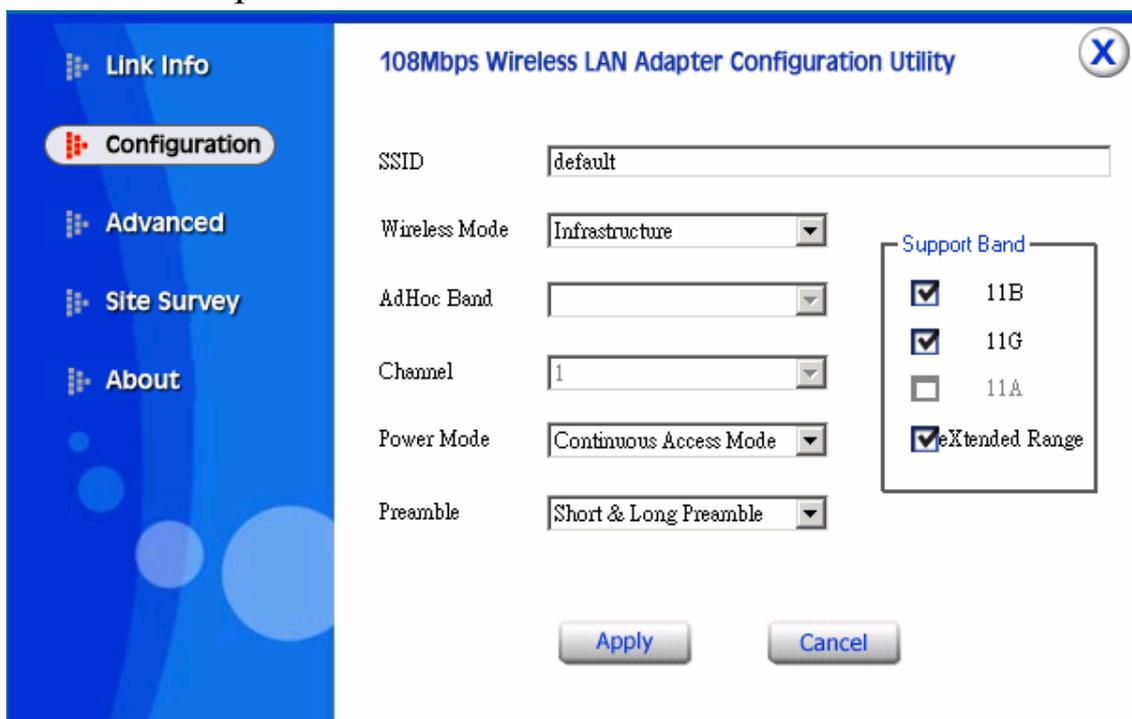
**SSID:** Service Set Identifier, which is a unique name shared among all clients and nodes in a wireless network. The SSID must be identical for each clients and nodes in the wireless network.
