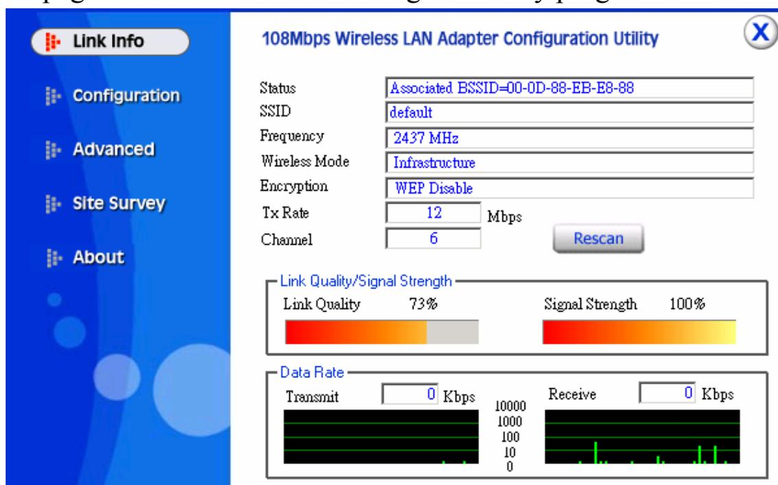
**Status:** Shows the BSSID associated, which can be used to identify the wireless network.
