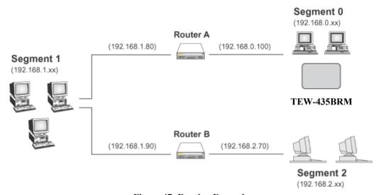
Figure 47: Routing Example
