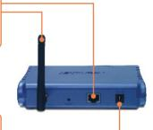
Connect the Power Adapter to the Access Point and then to a power outlet.
