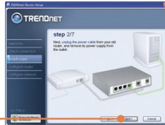
4. Disconnect the Ethernet cable from the port labeled "WAN" or "Internet" on the back of your old router. Plug this cable into the grey port labeled "WAN" on the TEW-432BRP. Then click **Next**.
