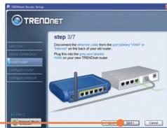
5. Disconnect all remaining Ethernet cables from the back of your old router and plug them into the yellow ports on the TEW-432BRP.
