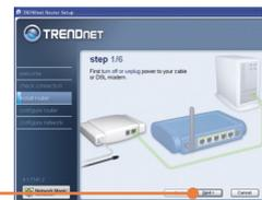
8. Unplug the existing Ethernet cable from your cable or DSL modem and plug it into yellow port number 1 on the TEW-432BRP. Then click **Next**.
