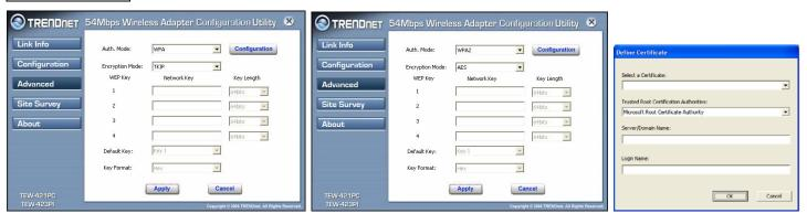
If WPA or WPA2 is selected, the above screen is shown. Please select the encryption type from the drop down menu and press *Configuration* to setup parameters for the RADIUS server.
