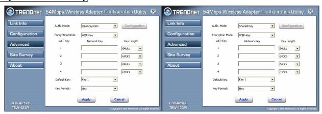
**WEP Key 1~4**: choose the encryption, either in HEX or ASCII formats, and enter the password in the blank space.
