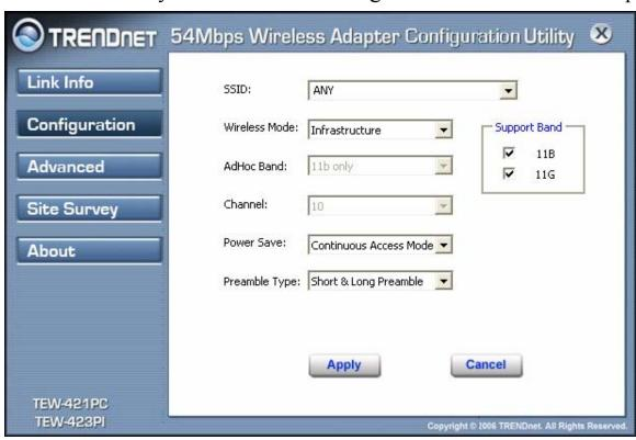
**SSID:** Service Set Identifier, which is a unique name shared among all clients in a wireless network. The SSID must be identical for each client and node in the wireless network.
