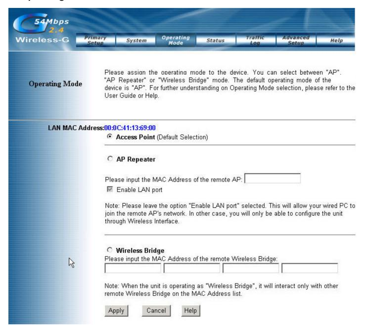
**Access Point:** This mode provides access for wireless stations to wired LANs and from wired LANs to wireless stations.
