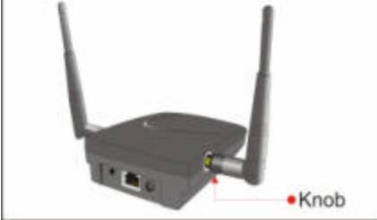
**4** The antenna should fit securely in place.
