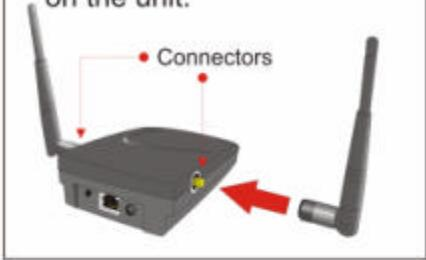
**3** Screw in antenna by turning the knob clockwise.
