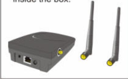
**2** Locate antenna connectors on the unit.
