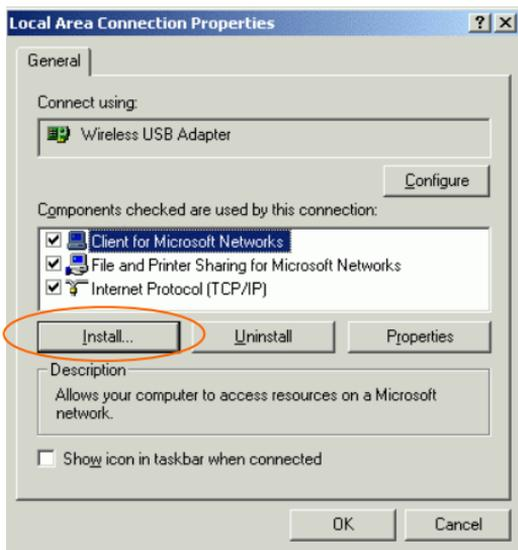
3. If any components are missing, click on the **Install...** button to select the **Client/Service/Protocol** required. After selecting the component you need, click **Add...** to add it in
