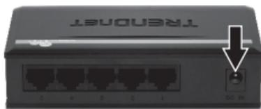
2. Connect a Cat.5e or Cat.6 RJ-45 network cable from the computer to an available Ethernet port on the TEG-S5g.
