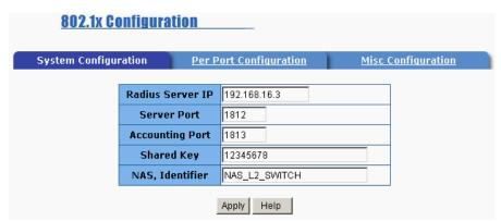
802.1x Configuration - System Configuration interface
