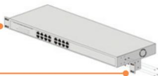
4. Carefully position the chassis onto the rack. Align the bracket to the screw holes on the rack, then use the screws provided with the equipment rack to mount the chassis.
