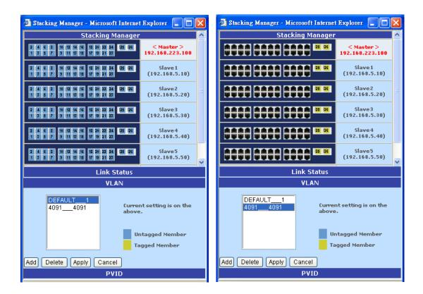
As seen above, the VLAN name "DEFAULT" and VID "1" is standard setting for general Tag VLAN, and all port are added as untagged port; The other VLAN "4091", as so called "Stacking Tag VLAN", is an unique setting for this type of stacking. And all of their Giga ports are set to tag members to form a VLAN connection channel.
