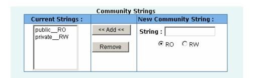
**3. Trap Manager**: A trap manager is a management station that receives traps, the system alerts generated by the switch. If no trap manager is defined, no traps are issued. Create a trap manager by entering the IP address of the station and a community string.
