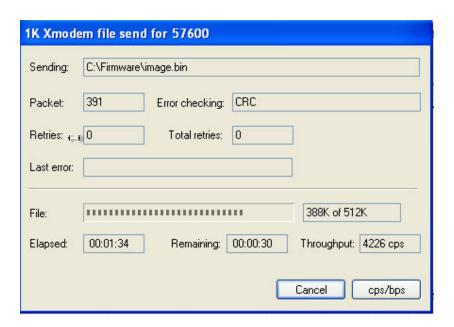
5. After firmware downloading already, the switch will update firmware automatically. After that, the switch will reboot.
