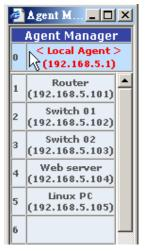
The agent manager holds 32+1 slots in the floating menu. The most top slot (zero slot) displays the master switch IP and its relative location. "Remote Agent" means that the user comes from the other IP domain than the managed ones, while "Local Agent", that user comes form the same one as the managed ones.
