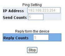
This page will display the result of the pinging IP. It continues updating the "Reply Counts" when the ping packets are sending. User can interrupt the progress by clicking "Stop" button.
