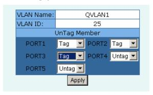
7. Uses this page to set the outgoing frames are VLAN-Tagged frames or no. Then click Apply.
