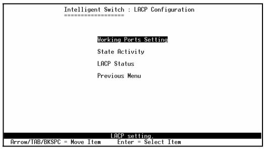
**Note:** All ports support LACP dynamic trunk group. If connecting to the device that also supports LACP, the LACP dynamic trunk group will be created automatically.
