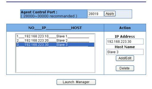
**Agent Control Port:** The control port defines the specific TCP/UDP port the single IP switch is listening, which the agent manager sends its command to. Agent manager use this specific port to tell single IP switch to change the current forwarding target host. The range of available port number is 28000 ~ 30000. Ignore the default settings of "Agent Control Port" unless user has the special need for this protocol port, such as virtual server. The default port number is 28019.
