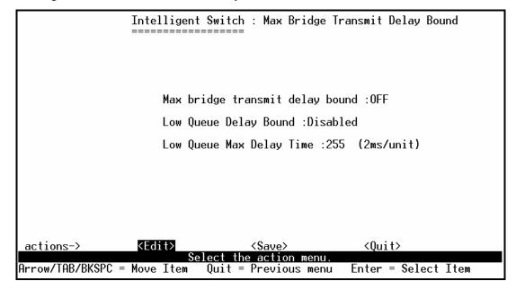
**NOTE:** Make sure "Max bridge transit delay bound control" is enabled before enabling Low Queue Delay Bound, because Low Queue Delay Bound must be work under "Max bridge transit delay bound control" is enabled situation.
