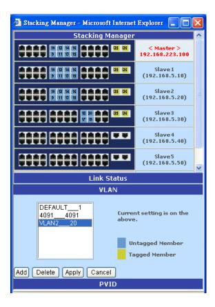
To delete a VLAN is also an easy task. Select the unwanted VLAN and press " Delete" to remove it.
