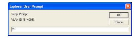
After input, user can choose the VLAN member in the Stacking Manager panel by clicking the designated port. Color cycling from blue, yellow to black means that the port is set to untagged port, tagged port or no member. When finishing, press "Apply" to submit.
