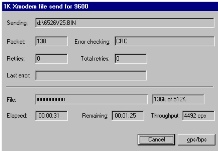
5. Finish download image, the switch system will update firmware automatic. Update firmware ok, the switch will reboot. Please change the Baudrate to 9600bps.
