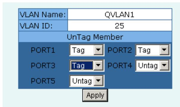
7. Uses this page to set the outgoing frames are VLAN-Tagged frames or no. Then click Apply.
