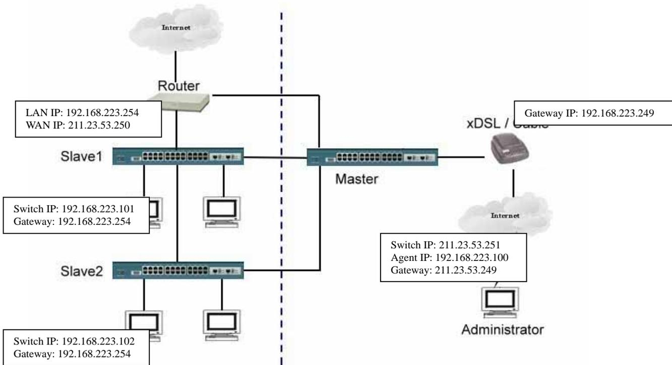
There are practical applications on combination of virtual server and single IP. Network administrator prefers a router as unique gateway to Internet while he/she likes to use the “Single IP” to manage the network both from LAN and WAN. This example gives a guide on how to setup virtual server with agent/stacking switch.
