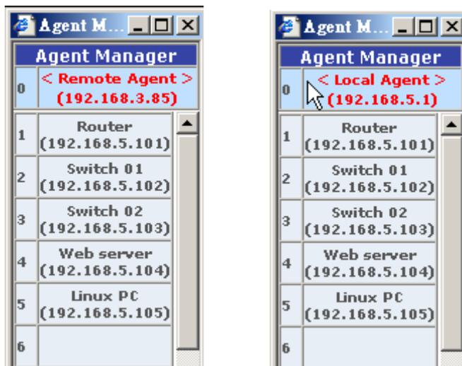
The agent manager holds 32+1 slots in the floating menu. The most top slot (zero slot) displays the master switch IP and its relative location. “Remote Agent” means that the user comes from the other IP domain than the managed ones, while “Local Agent”, that user comes from the same IP domain as the managed ones.
