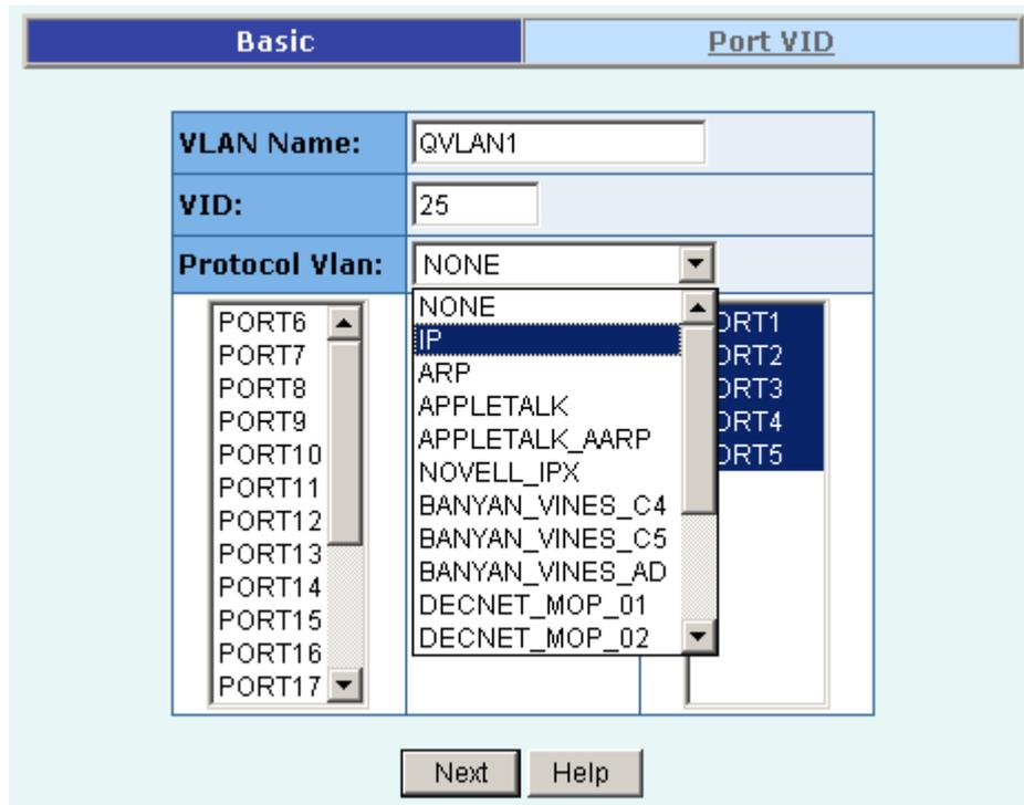
5. From the Available ports box, select ports to add to the switch and click “Add >>”. If the trunk groups exist, you can see it in here (ex: TRK1, TRK2...), and you can configure it is the member of the VLAN or not.
