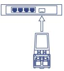
**Fiber Applications** Long distance fiber networking for manufacturing, business parks, and school campus applications. **Fiber Mode/Distance** Multi-Mode transceiver spans distances up to 550m (1804 ft.) at gigabit speeds.
