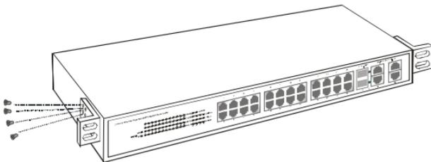
**Figure 2. Combine the Switch with the provided screws**
