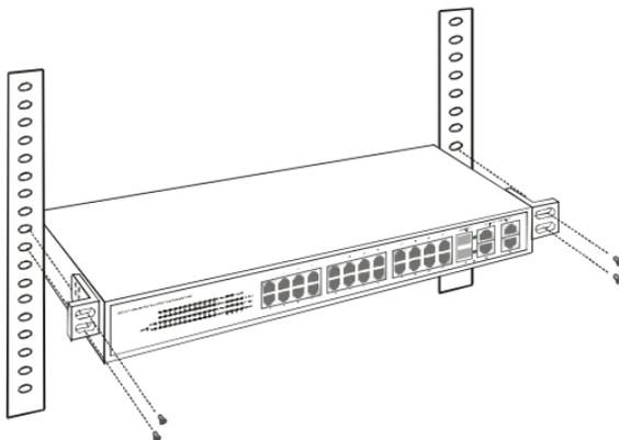
**Figure 3. Mount the Switch in the rack**
