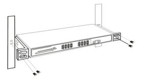
Figure 3. Mount the Switch in the rack
