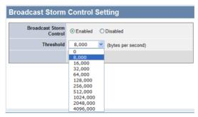
Figure 42. Broadcast Storm Control Setting
