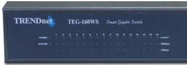
Figure 6. LED indicators of the Switch
