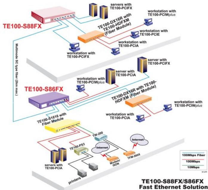
TE100-S88FX/S86FX Fast Ethernet Solution
