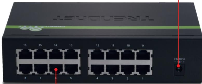
2. Connect a CAT-5, CAT-5e or CAT-6 RJ-45 network cable from the computer to an available Ethernet port on the TE100-S16Eg
