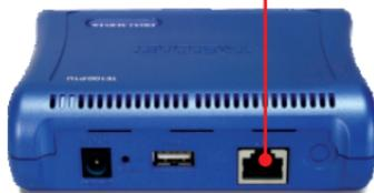
2. Connect the USB Printer to the USB port of the Print Server.
