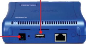
3. Connect the Power Adapter to the Print Server and then to a power outlet.
